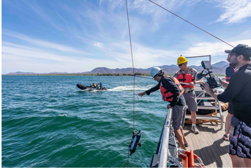
Deploying a CTD in the Gulf of California, April 2025. Photo Credit: Patrick Webster.
